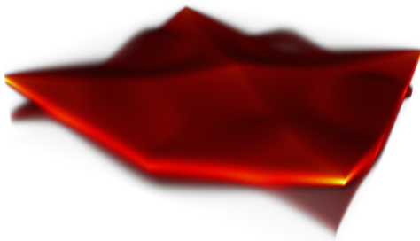
Figure 10: Volume rendering of a hixel data set generated by sampling images 3200 values sampled from a Poisson distribution and 9600 values sampled from a normal distribution. There are 512x512 hixels in this data set, each with 128 bins. The shortest axis in the images corresponds to histogram bins, thus a spatially higher location along that axis indicates a higher function value. Color and opacity are used to illustrate the density of the samples. Thus the lower, right corner of shows a hixel with 2 distinct probable function values; the smaller function value is less probable than the larger.
